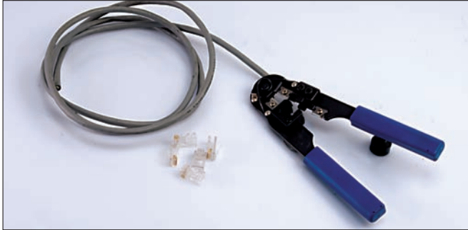
This is all you need to start crimping your own network cables.
